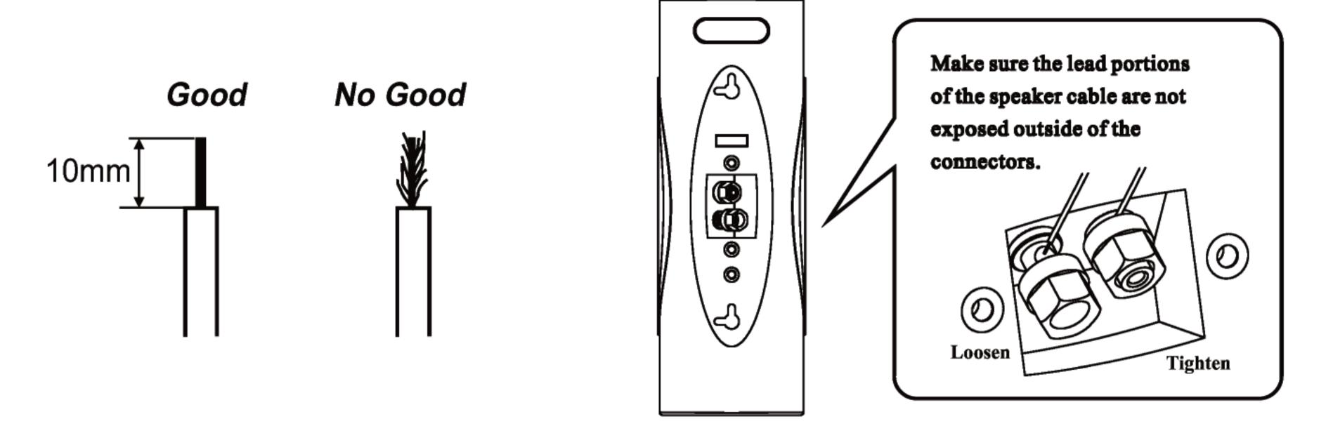
③ Tighten the knob and secure the cord. Test the firmness of the connection by pulling lightly on the cord at the terminal.
